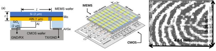
(b) Ultrasonic fingerprint sensor
